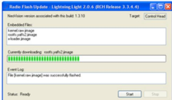
5. While holding the push-to-talk on the microphone connected to the remote control head, turn on radio power. (Note: The radio must be connected to the computer before power-up.)
