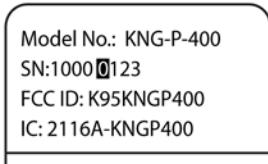
5000 Channel, P25 Trunking Capable/Upgradable version will display the BK Technologies logo at power-up and have a "9" as the fifth digit in the serial number.
